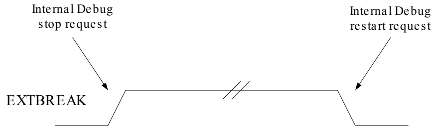
Figure 8-1. External BREAK output signal level on internal stop and restart request
