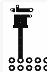
Figure 5. Minimum Pads of 2-ounce Copper
