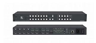
The VS-62HA is a high-quality matrix switcher for 4K UHD HDMI and analog audio signals that employs advanced auto switching schemes and control options. It reclocks and equalizes the signals and can route any input to either or both outputs simultaneously. It supports resolutions up to 4K@60Hz (4:2:0) UHD and WUXGA.
