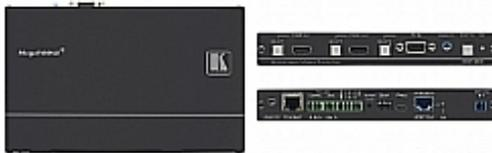
The DIP-20 is a 4K UHD, HDBaseT transmitter and Step-in commander for computer graphics video, HDMI, unbalanced stereo audio signals embedding and de-embedding. The DIP-20 accepts HDMI and PC graphics video input, an Ethernet signal, serial data, and an unbalanced stereo audio input (that is embedded into the output signal). It transmits the signal via HDBaseT (twisted pair) cable to a compatible receiver (for example, the TP-588D or TP-580RXR).
