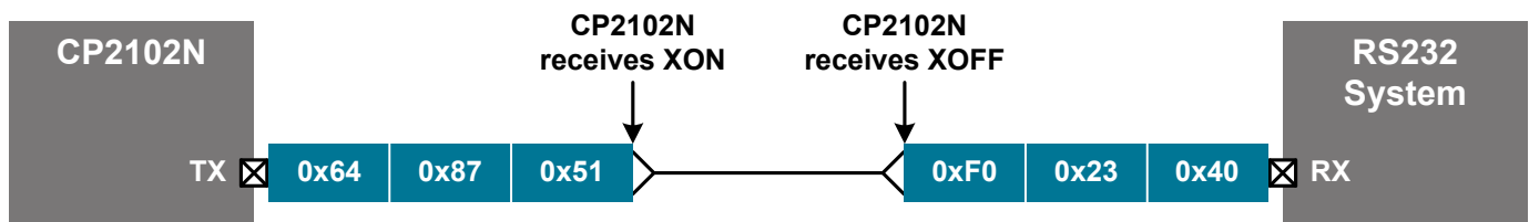
Figure 4.2. Software Flow Control Timing Diagram
