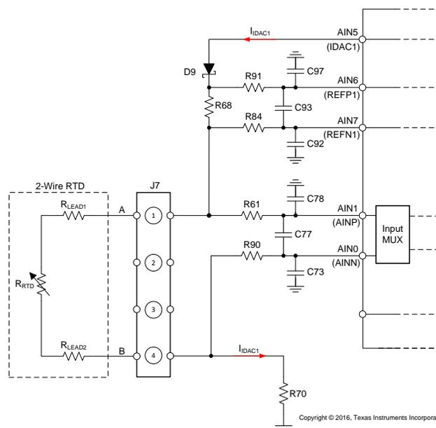
Figure 15. Simplified 2-Wire RTD Input Diagram
