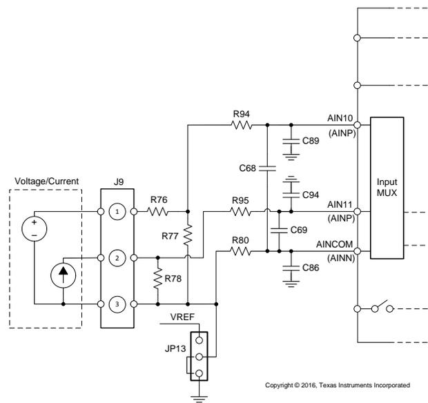
**Figure 21. Simplified Voltage and Current Input Diagram**
