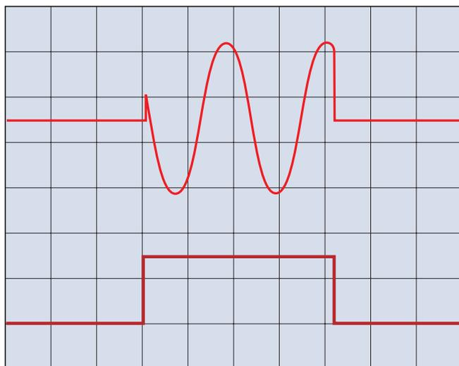
Fig. 7.2: Output signal controlled by a GATE signal
