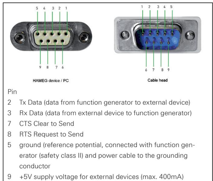
Fig. 8.1: Pin assignment of the RS-232 interface
