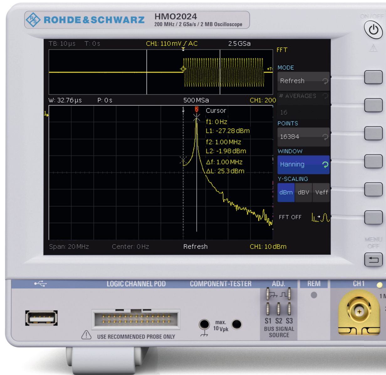
Figure 5: FFT analysis of a sine burst signal with Hanning window function
