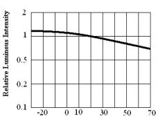
$\label{eq:ambient} \begin{tabular}{ll} Ambient Temperature $Ta$= $^{\circ}$C \\ Luminous Intensity vs. Ambient Temperature \\ \end{tabular}$
