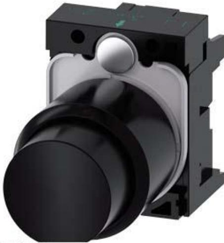
PUSHBUTTON, COMPACT, WITH EXTENDED STROKE (12MM), 22MM, ROUND, PLASTIC, BLACK, RAISED BUTTON, MOMENTARY CONTACT TYPE, WITH HOLDER
