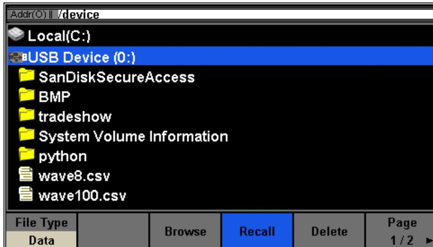
Figure 26- Load an Arb Waveform from External USB
