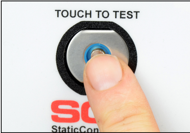
Figure 7. Bridging the test switch's contacts to initiate the test
