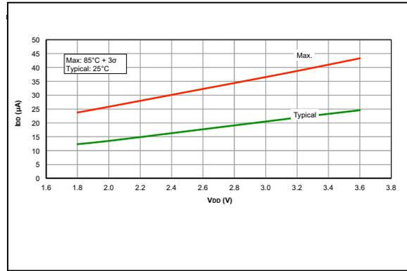
**FIGURE 26-4:**  $I_{DD}$ , EC Oscillator, Low-Power mode,  $F_{osc} = 500$  kHz
