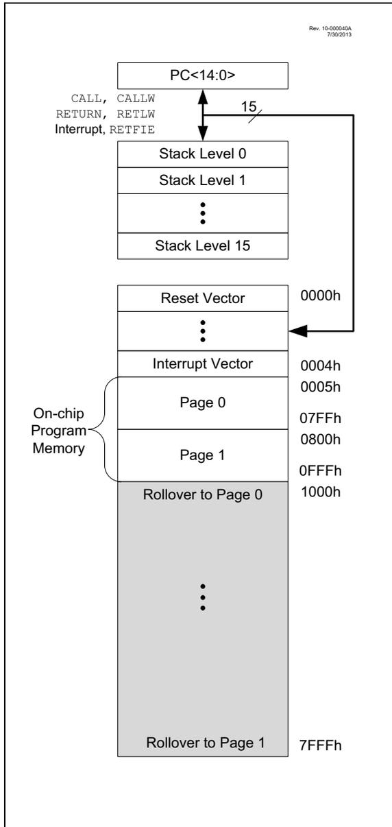
**FIGURE 3-2: PROGRAM MEMORY MAP AND STACK FOR PIC16LF1559**
