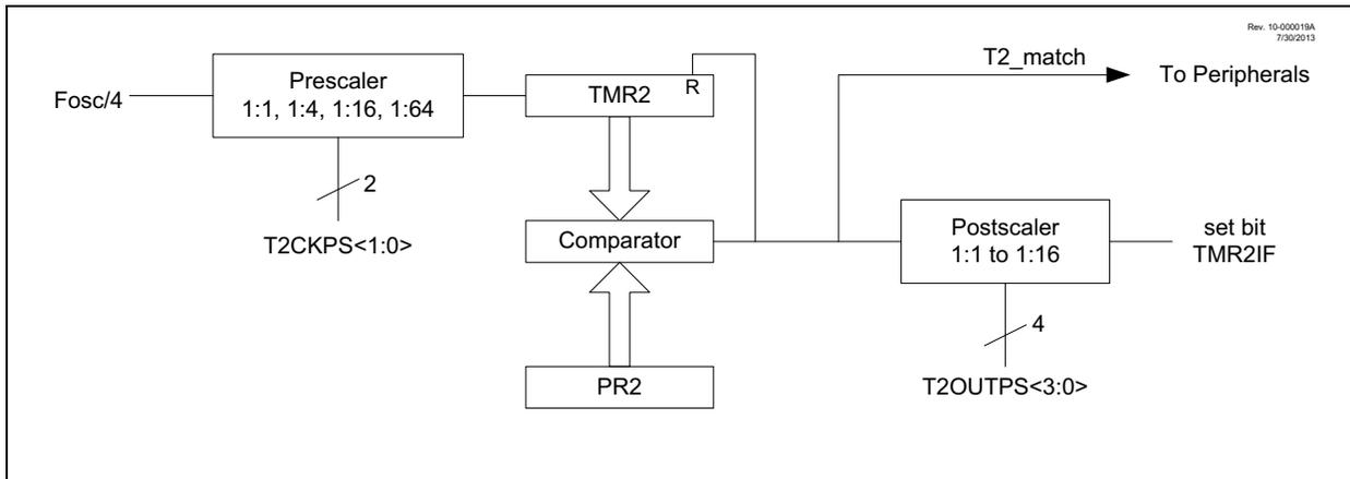
**FIGURE 19-2: TIMER2 TIMING DIAGRAM**
