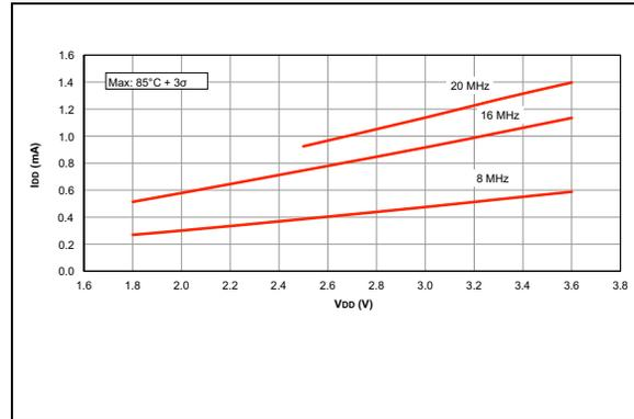
**FIGURE 26-6:**  $I_{DD}$  Maximum, EC Oscillator, High-Power Mode
