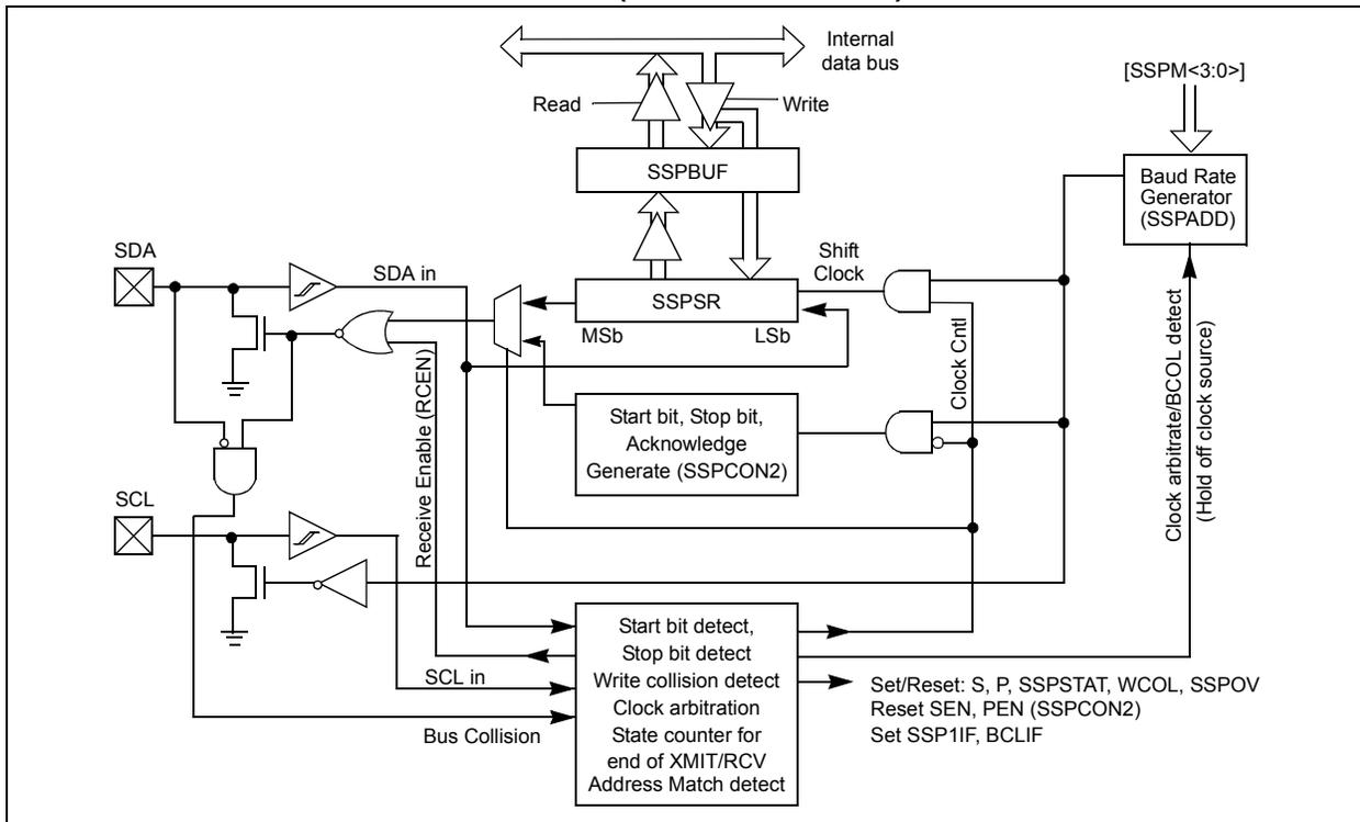
**FIGURE 20-3: MSSP BLOCK DIAGRAM (I<sup>2</sup>C SLAVE MODE)**
