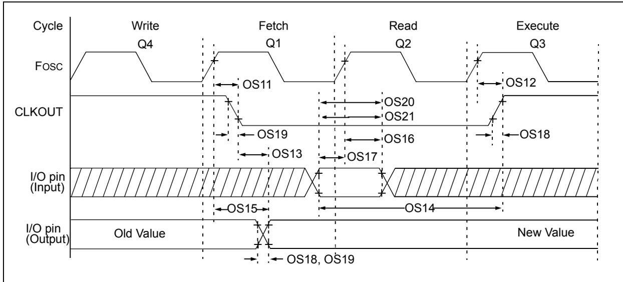
**TABLE 25-9: CLKOUT AND I/O TIMING PARAMETERS**
