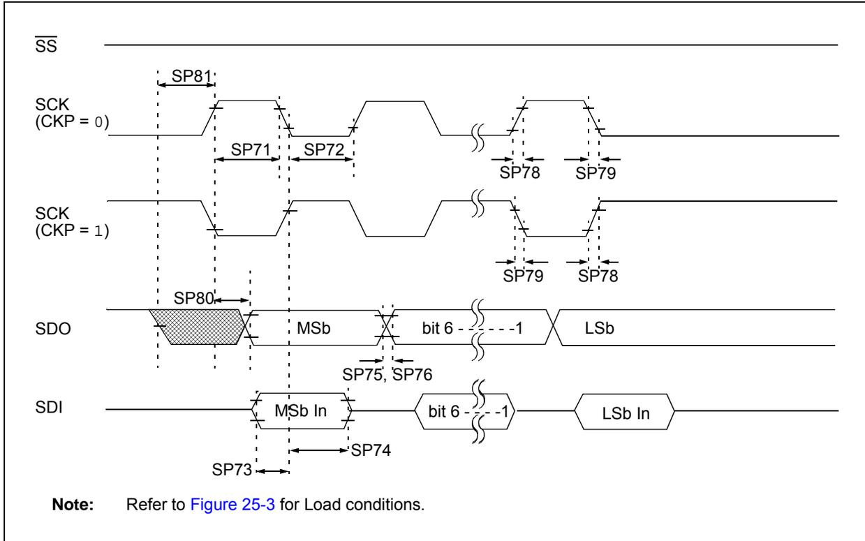
**FIGURE 25-14: SPI MASTER MODE TIMING (CKE = 1, SMP = 1)**
