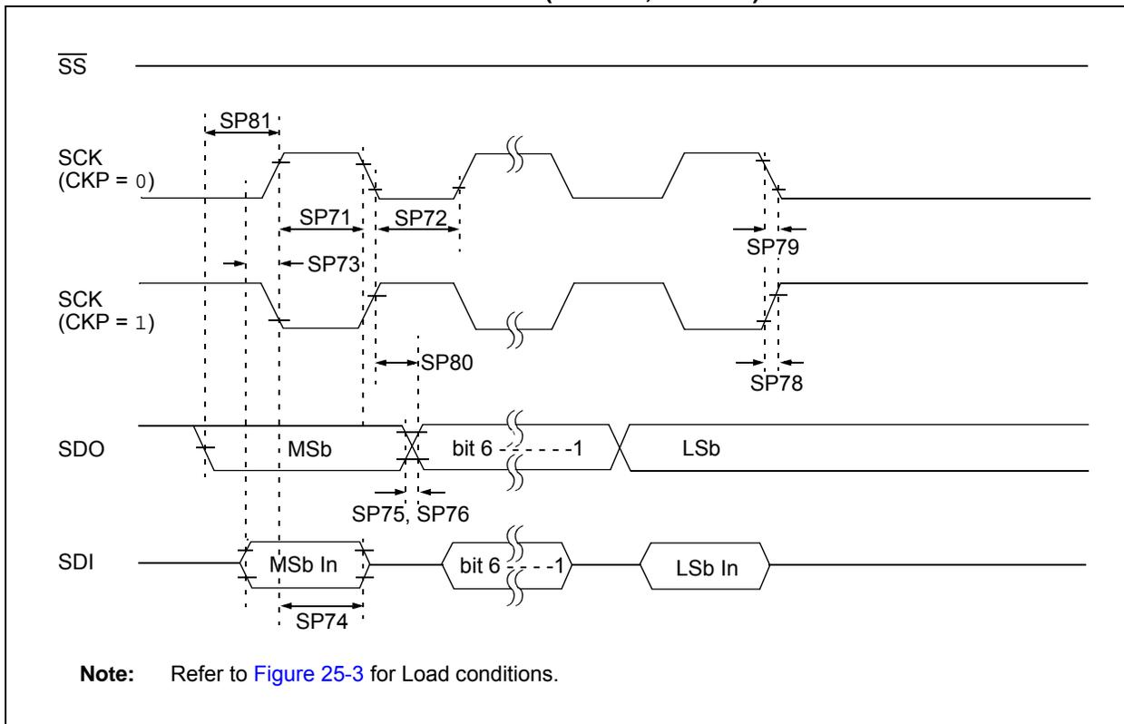
**FIGURE 25-15: SPI SLAVE MODE TIMING (CKE = 0)**
