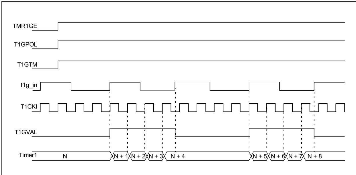
**FIGURE 18-5: TIMER1 GATE SINGLE-PULSE MODE**
