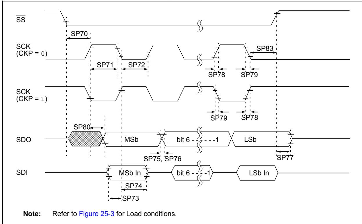
**FIGURE 25-16: SPI SLAVE MODE TIMING (CKE = 1)**
