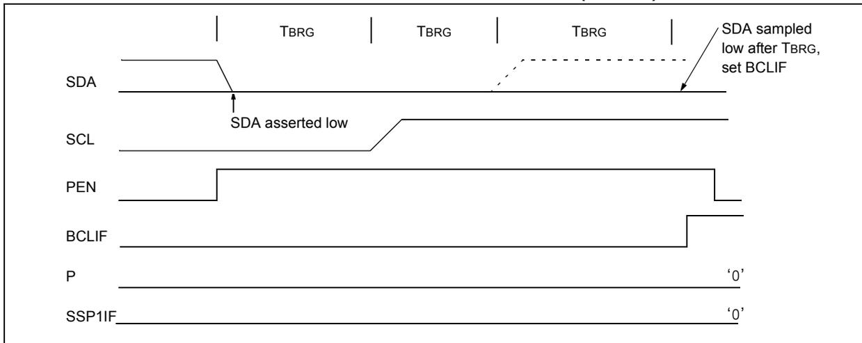
**FIGURE 20-39: BUS COLLISION DURING A STOP CONDITION (CASE 2)**
