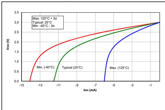
**FIGURE 26-14:**  $V_{OH}$  vs.  $I_{OH}$ , over Temperature,  $V_{DD}=3.0V$
