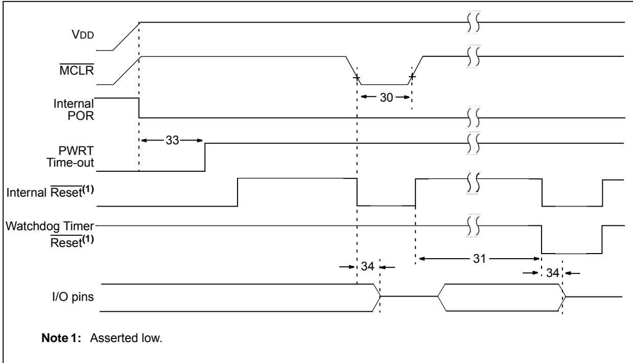
**FIGURE 25-7: BROWN-OUT RESET TIMING AND CHARACTERISTICS**
