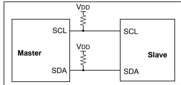
The Acknowledge bit ( $\overline{\text{ACK}}$ ) is an active-low signal, which holds the SDA line low to indicate to the transmitter that the slave device has received the transmitted data and is ready to receive more.
