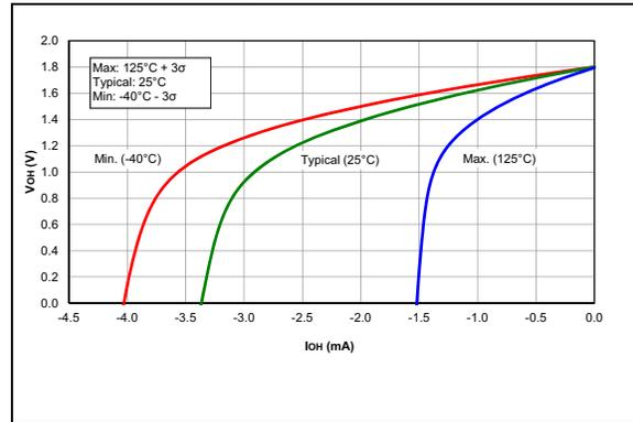
**FIGURE 26-16:**  $V_{OH}$  vs.  $I_{OH}$ , over Temperature,  $V_{DD}=1.8V$
