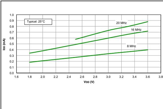
**FIGURE 26-3:**  $I_{DD}$  Typical, EC Oscillator, High-Power Mode
