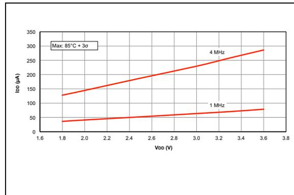
**FIGURE 26-5:**  $I_{DD}$  Maximum, EC Oscillator, Medium-Power Mode
