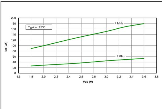
**FIGURE 26-2:**  $I_{DD}$  Typical, EC Oscillator, Medium-Power Mode
