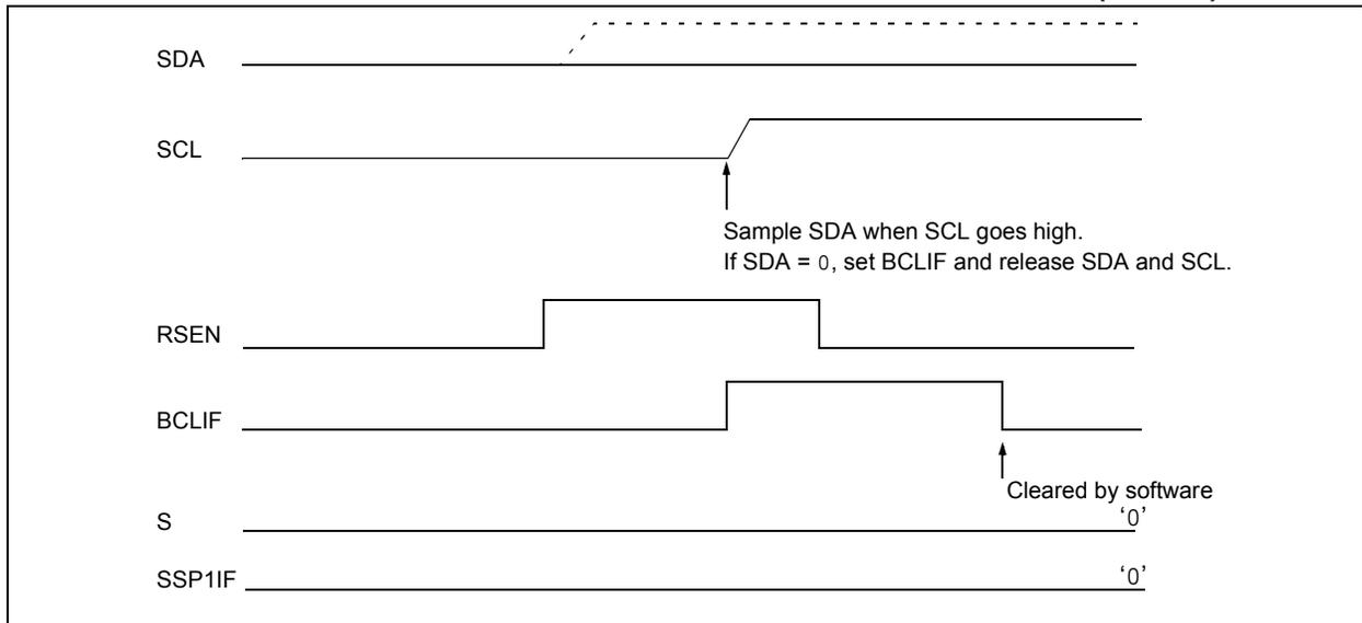
**FIGURE 20-37: BUS COLLISION DURING REPEATED START CONDITION (CASE 2)**
