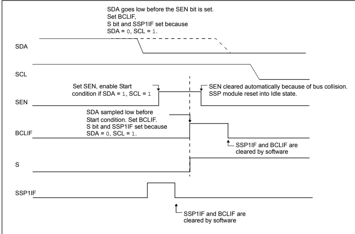
**FIGURE 20-34: BUS COLLISION DURING START CONDITION (SCL = 0)**
