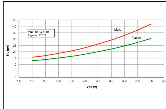
**FIGURE 26-12:**  $I_{PD}$ , Fixed Voltage Reference (FVR)
