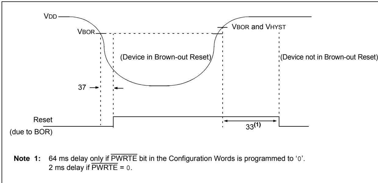
**TABLE 25-10: RESET, WATCHDOG TIMER, POWER-UP TIMER AND BROWN-OUT RESET PARAMETERS**
