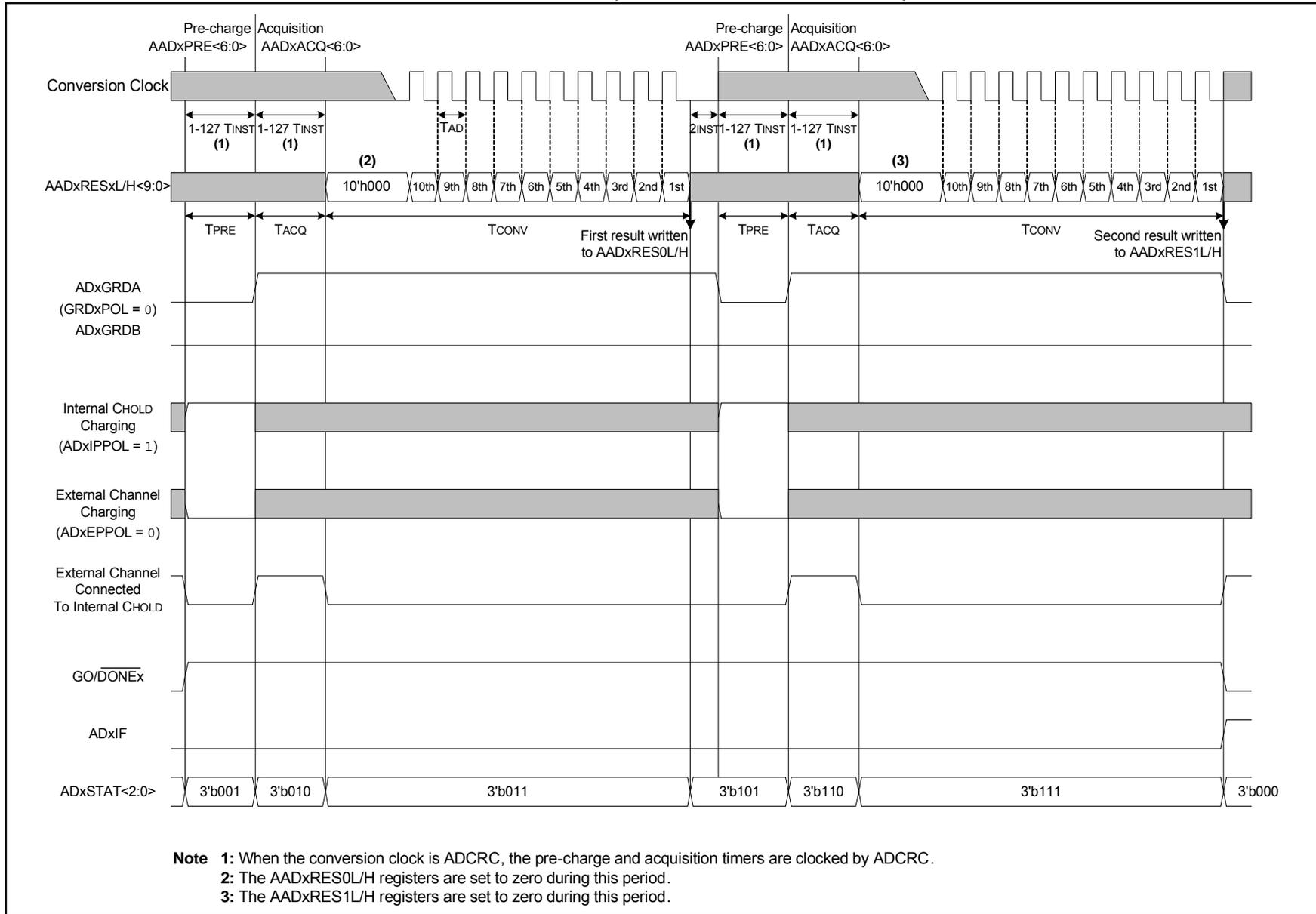
**FIGURE 16-7: DOUBLE SAMPLE CONVERSION SEQUENCE (ADDSSEN = 1 AND ADIPEN = 1)**
