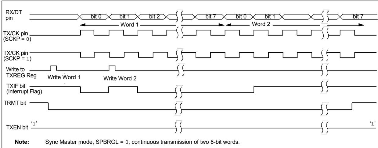
**FIGURE 21-11: SYNCHRONOUS TRANSMISSION (THROUGH TXEN)**
