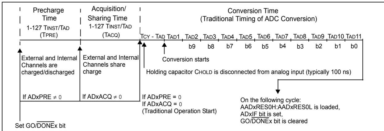
**FIGURE 16-6: DOUBLE SAMPLE CONVERSION SEQUENCE (ADDS<sub>EN</sub> = 1 AND ADIPEN = 0)**
