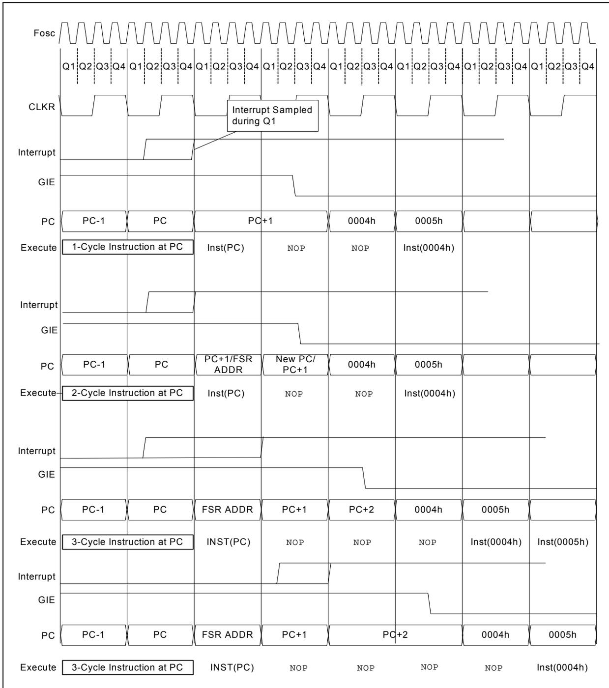
**FIGURE 7-3: INT PIN INTERRUPT TIMING**
