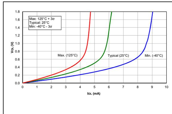
**FIGURE 26-17:**  $V_{OL}$  vs.  $I_{OL}$ , over Temperature,  $V_{DD}=1.8V$
