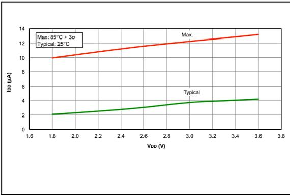
**FIGURE 26-1:**  $I_{DD}$ , EC Oscillator, Low-Power mode,  $F_{osc}=32$  kHz
