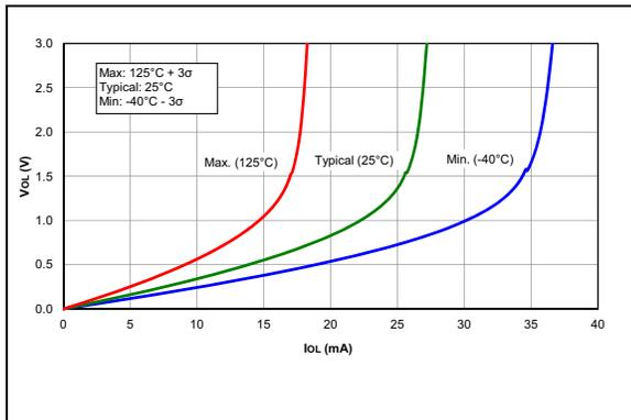
**FIGURE 26-15:**  $V_{OL}$  vs.  $I_{OL}$ , over Temperature,  $V_{DD}=3.0V$
