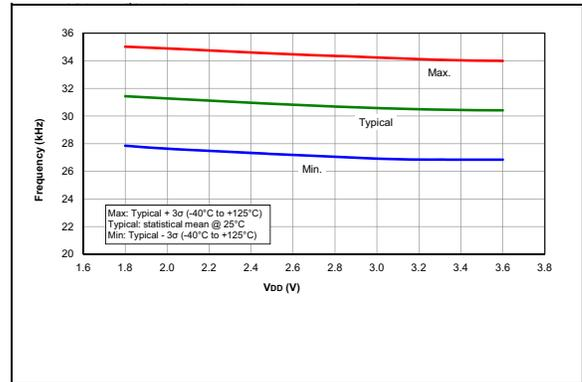
**FIGURE 26-22:** LFINTOSC Frequency over  $V_{DD}$  and Temperature
