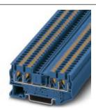
Feed-through terminal block, Connection method: Push-in connection, Cross section: 0.14 mm² - 4 mm², AWG: 26 - 12, Width: 5.2 mm, Height: 35.3 mm, Color: blue, Mounting type: NS 35/7,5, NS 35/15
