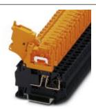
Disconnect terminal block, Connection method: Spring-cage connection, Cross section: 0.08 mm² - 6 mm², AWG: 28 - 10, Width: 6.2 mm, Color: black/orange, Mounting type: NS 35/7,5, NS 35/15
