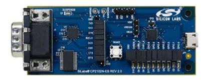
The CP2102N-EK kit is designed to showcase the various features of the <u>CP2102N USBXpress</u> <u>devices</u>. These highly-integrated USB-to-UART bridge controllers provide a simple solution for updating RS-232 designs to USB using a minimum of components and PCB space. By eliminating the need for complex firmware and driver development, the CP2102N devices enable quick USB connectivity with minimal development effort.
