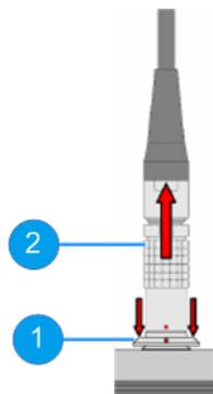
**Fig. 3-3: Disconnecting the host connector**
