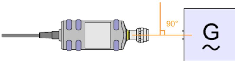
3. To ensure a maximal measurement accuracy, tighten the RF connector using a torque wrench with the recommended nominal torque (see the operating manual of your power sensor).
