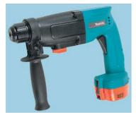
12V cordless SDS-Plus rotary hammer drill. Features include easy bit changeover facility, 3-mode switch (rotation only, rotation with hammer and hammer only), forward and reverse switch, variable speed control and built-in torque limiter. Standard equipment includes depth gauge, 2 x 2.0Ah Ni Cd battery packs, charger, side handle and carrying case.
