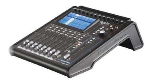
all the analogue electronics and analogue I/O are placed in the short section and are therefore shielded from the digital electronics, screens and (in the case of the digiLive) moving fader motors, which occupy the longer arm. The triangular gap between the tabletop and the bottom of the casing allows for convection cooling and removes the need for an internal fan.
