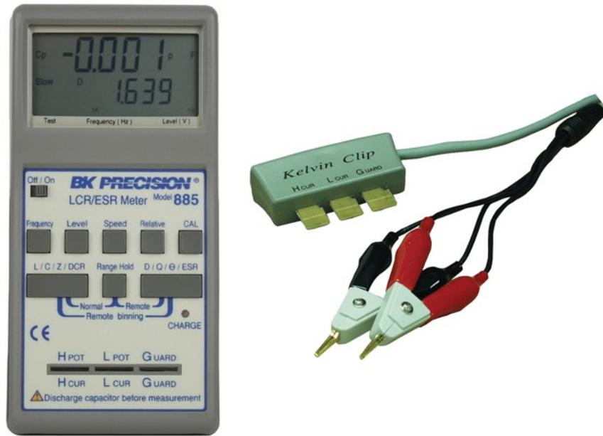
Figure 14: 885 LCR meter with Kelvin clips
