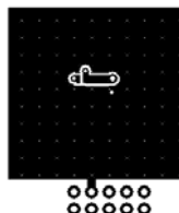
a. 53^\circ\text{C}/\text{W} when mounted on a 1 in 2 pad of 2 oz copper
