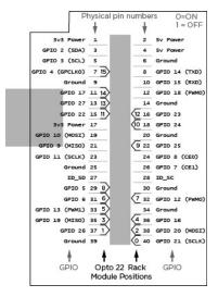
Place this overlay over your Pi's GPIO pins for a handy mapping reference. You can download the template from developer.opto22.com.
