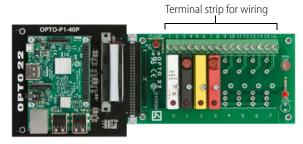
**7.** Follow "Field Wiring Diagrams" on page 4 to wire realworld sensors and devices to the mounting rack.
