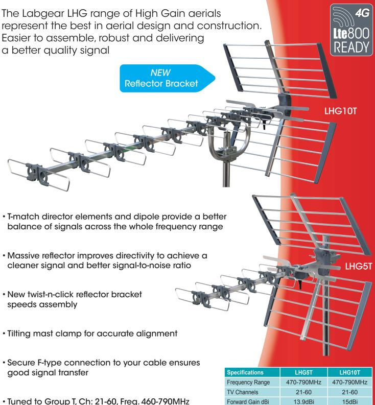
LHG aerials are supplied in an individual box with tilting mast clamp, f-connector, rubber weather boot and installation guide. For improved stability the larger LHG10T is supplied with a centre bracket.
