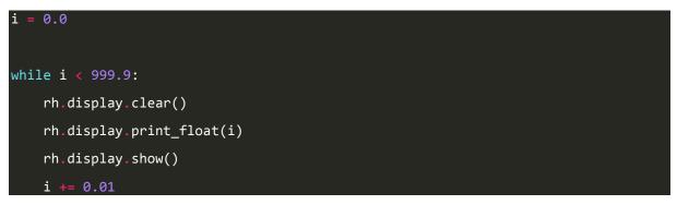
This starts at 0.0, clears the display, then uses the print\_float method and show to display the current value of i, and finally increments i by 0.01.
