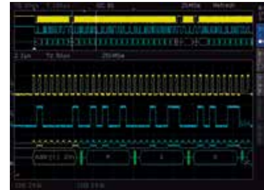
SPI bus signal, MISO / MOSI decoded
