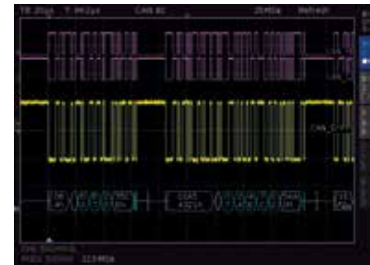
HEX decoded CAN bus signal
