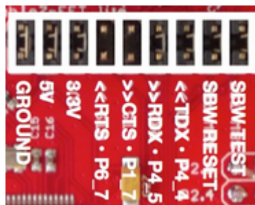
Figure 33. eZ-FET or eZ-FET Lite Debug Connector
