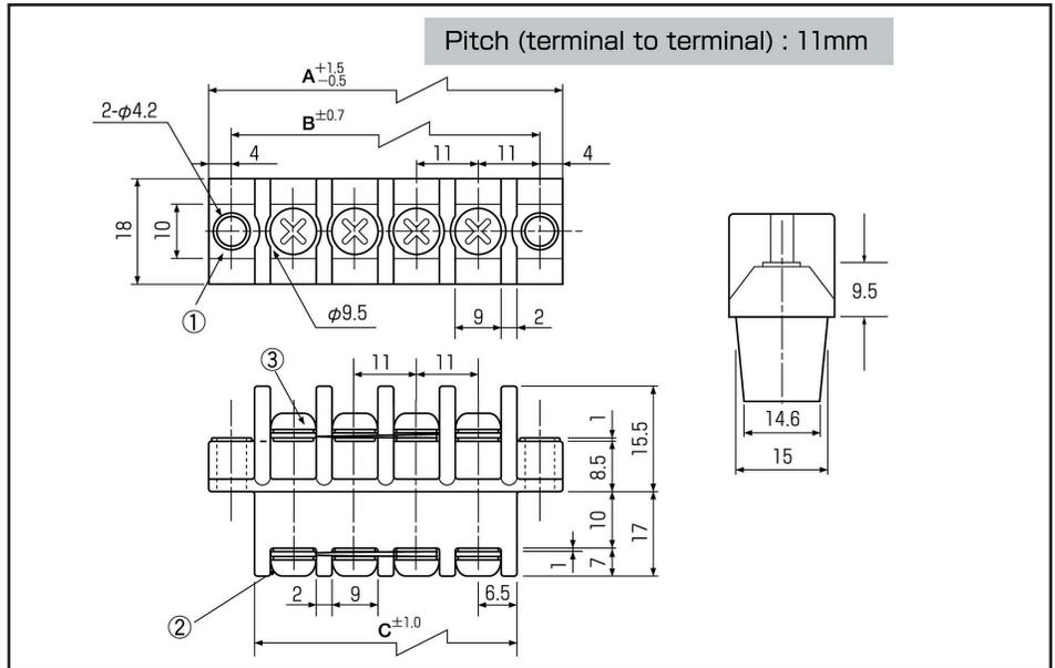
BlockMaster Electronics' new OGM-300NE Series are medium power, thru-panel terminal blocks available in 2-23 positions.
