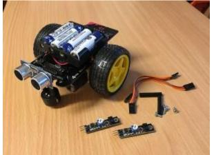
30mm black nylon M3 pillars 6mm M3 screws x 4 Line follower sensors x 2 10cm GVS cables x 2
