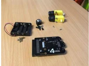
Fit 4 of the 8mm M2.5 CSK screws and the 4 nuts to the Robo:Bit as shown above. Pass each screw from the top of the board into a nut on the bottom. Tighten securely.
