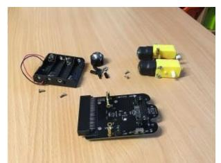
Using 2 of the 6mm M2.5 pan head screws, fit the 11mm brass pillars in place for the 4-cell battery holder – the outermost two holes – as shown above. Tighten securely
