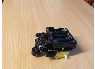
Use the remaining 2 of the 8mm M2.5 CSK screws to screw the battery holder to the brass mounting pillars.
