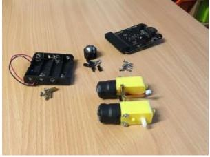
Place the motors into position as shown above, with the axles facing outwards Use 2 of the 25mm screws to fit the M3 black nylon 25mm female-female spacer to the bottom holes in the motor
