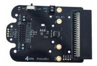
Robo:Bit is a general purpose robotics controller for the BBC Micro:Bit, that also converts easily into a self-contained little buggy.
