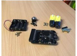
Robo:Bit Battery Holder Yellow gear motors x 2 1 caster (metal ball plus plastic housing) 10mm black nylon male-female pillars x 2 15mm black nylon female-female pillars x 2 25mm black nylon female-female pillar (M3) 25mm brass female-female pillars x 2 25mm M3 screws x 4 6mm M2.5 screws (pan head) x 8 8mm M2.5 screws (CSK) x 6 M2.5 nuts x 4 4-cell AA battery holder
