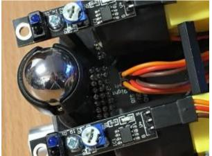
Pass the wires around the motor supports and then into the 3×2 male header underneath the Robo:Bit board. Make sure brown goes to Ground (GND), Red to power (3V) and Orange to Signal (SIG)
