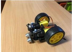
Push one of the GVS leads onto each line follower sensor. Make sure you use the colour coding: Brown for Ground (G), Red for volts (V+) and Orange for Signal (S) Then use the remaining 2 of the 6mm M3 screws to to fit the line sensors to the bottom of each pillar. Use the hole near the centre of the sensor, not the one at the front. The wires should be at the back, as shown above
