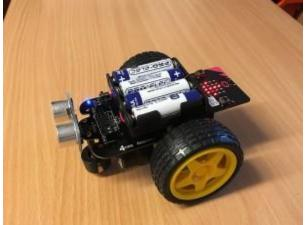
Push on the wheels. Be careful to hold the motor as the wheels can be quite stiff to fit, especially the first time Push in the Ultrasonic Sensor (if you have one)
