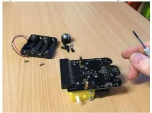
Use 2 of the 6mm M2.5 pan-head screws to attach the Robo:Bit to the upwards-facing connectors on the brass bracket assembly as shown above. Tighten securely. Push the JST plugs from the motors into the sockets underneath the Robo:Bit controller. The wires are short enough to stay tidy.
