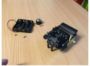
Screw each 10mm black nylon male-female pillar into a 15mm making it into a 25mm female-female pillar. Use a 6mm M2.5 pan-head screw to fit each pillar to the front holes on the Robo:Bit
