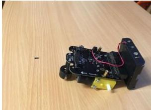
Screw the wires into the power terminal. Red to 5V and Black to GND. Wrap the wires tidily out of the way under the battery holder
