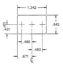
NOTE: A template can be made to these dimensions; or the 3 screw holes can be drilled (as per the instruction sheet) on these centers.
