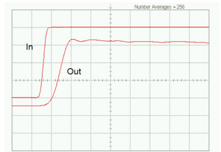
Typical response to 15 ps Rise time step
