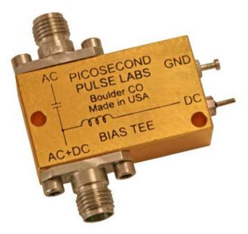
The PSPL5543 is an ultra-broadband, 500 mA current, coaxial bias insertion tee and 100 V DC blocking capacitor that passes high bandwidth pulses with very low waveform distortion. Its rise time is only 7 ps and its frequency response is flat over many decades from 20 kHz to beyond 50 GHz.
