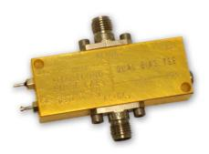
The PSPL5544 is an ultra-broadband, high-current, coaxial bias insertion tee and DC blocking capacitor. The high DC blocking voltage (100 V) and high bias current capability (2 A) make it an excellent choice for broadband measurements of power devices and circuits.
