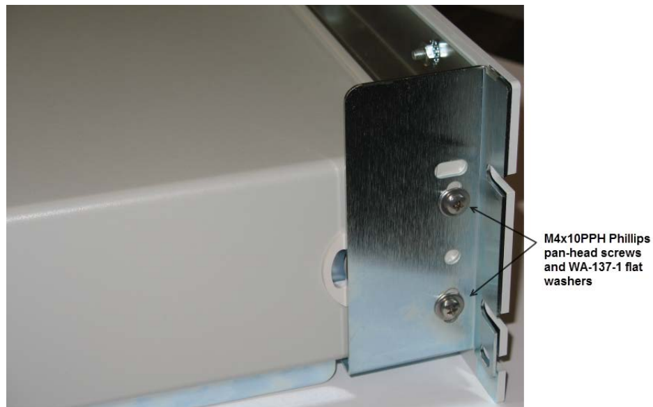
Figure 16: Rack-mount Series 2100 and Model 3390 instrument to chassis screws
