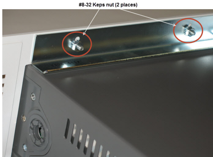
Figure 15: Model 4299-7 rack mount Series 2200 instrument to chassis bracket
