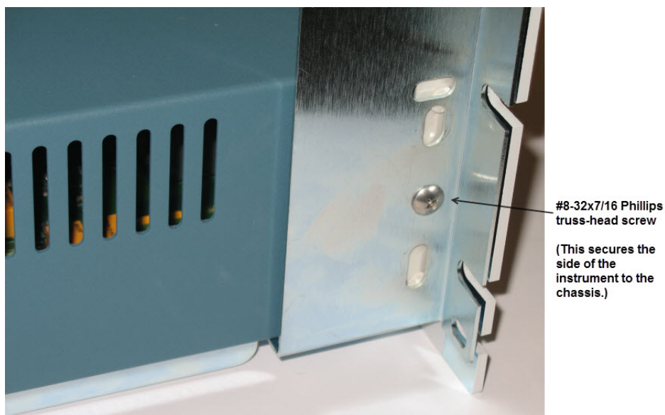
Figure 18: Rack-mount Tektronix DMM 4020, DMM 4040, DMM 4050 instrument to chassis screw
