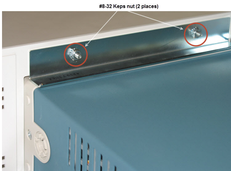
Figure 19: Rack-mount Tektronix DMM 4020, DMM 4040, DMM 4050 instrument to chassis Keps nut
