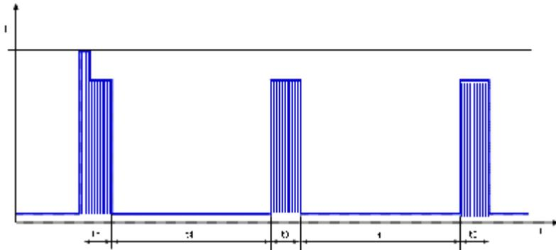
First pulse  $t_5$  typical 1,6s (1,3 .. 1,9s) followed by  $t_4$ . Afterwards cyclical  $t_3/t_4$ .
