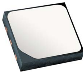
Figure 7. Si7007 with Factory-Installed Protective Cover
