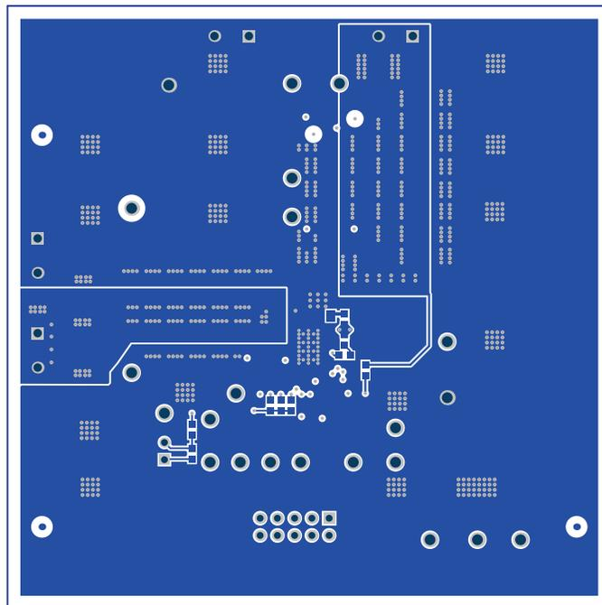
Figure 21. PWR-847EVM Bottom Layer (Top View)
