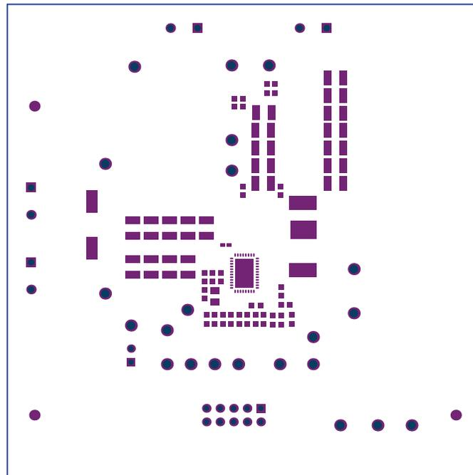
Figure 15. PWR-847EVM Top Solder Mask (Top View)
