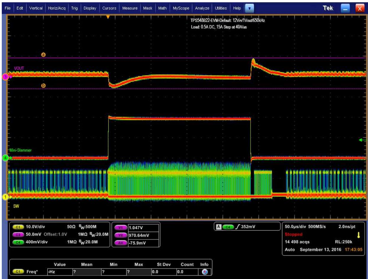
Figure 7. Transient Response of 1-V Output at 12 V<sub>IN</sub>, Transient is 0.5 A to 15.5 A, the Step is 15 A at 40 A/µs
