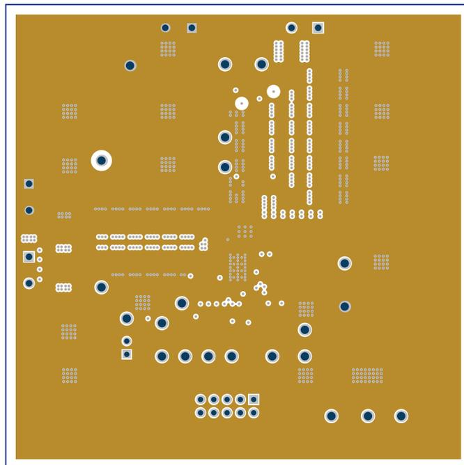
Figure 17. PWR-847EVM Inner Layer 1 (Top View)
