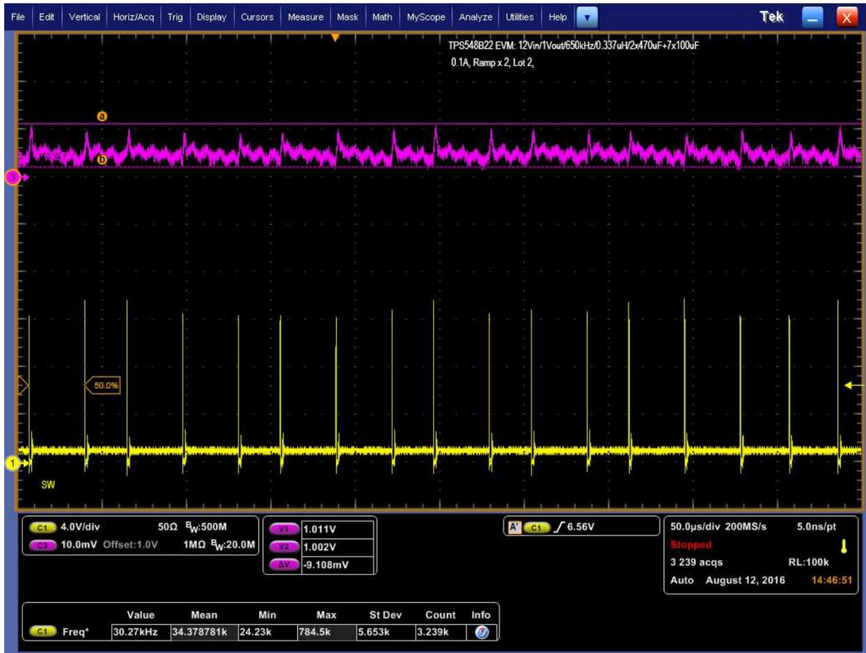
Figure 9. Output Ripple and SW Node of 1-V Output at 12 V<sub>IN</sub>, 0-A Output
