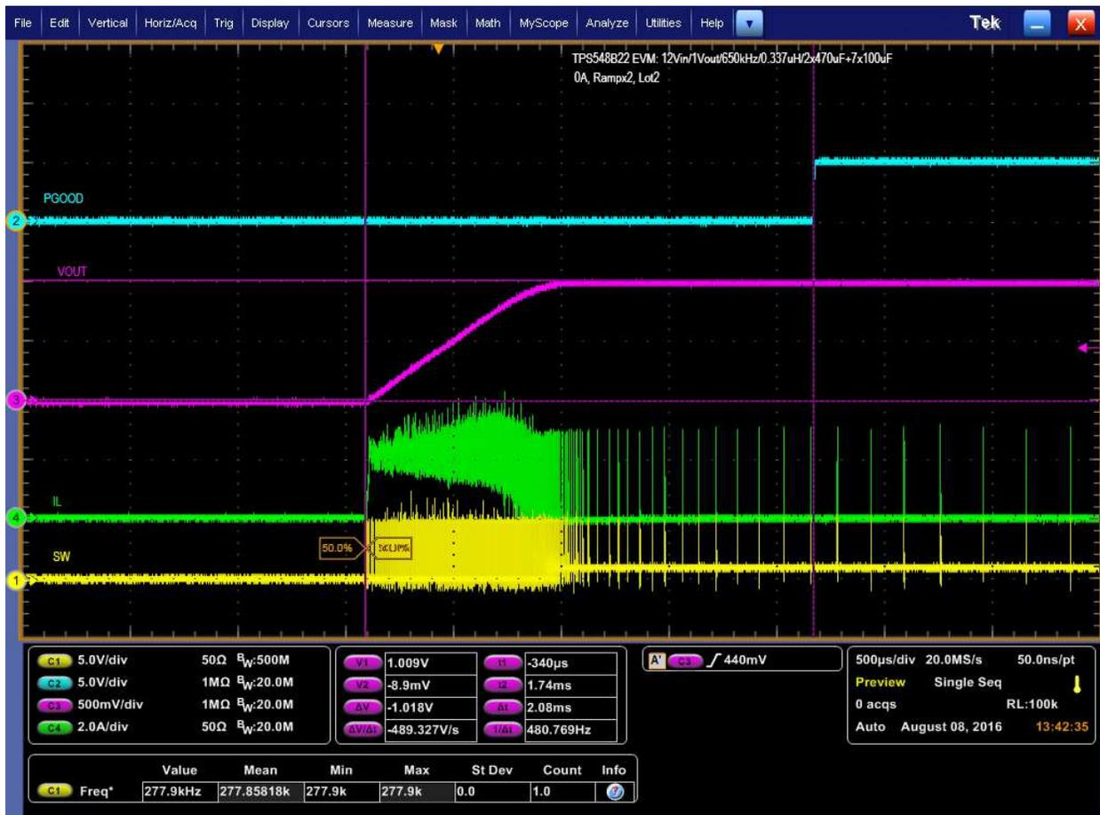
Figure 10. Start up from Control, 1-V Output at 12 V<sub>IN</sub>, 0-A Output
