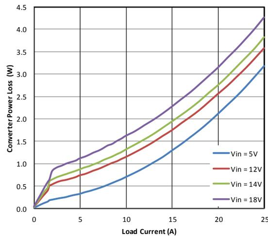
Figure 5. Power Loss of 1-V Output vs Load
