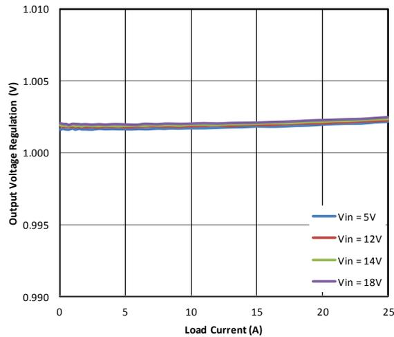
Figure 6. Load Regulation of 1-V Output
