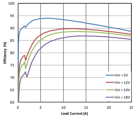
Figure 4. Efficiency of 1-V Output vs Load
