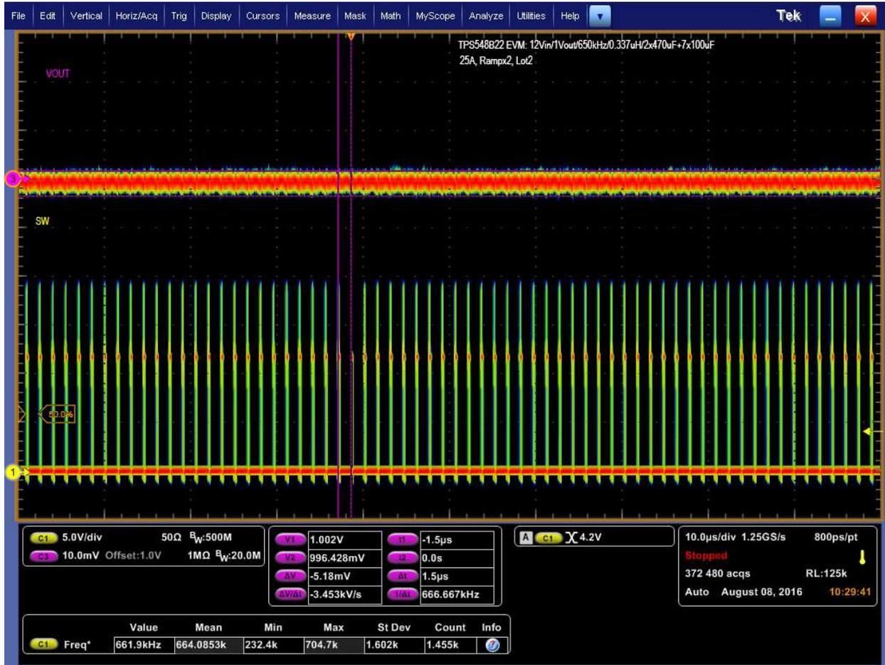
Figure 8. Output Ripple and SW Node of 1-V Output at 12 V<sub>IN</sub>, 25-A Output
