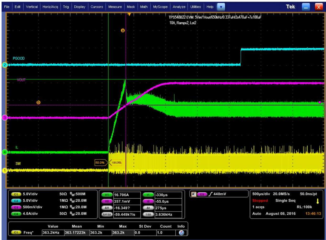
Figure 11. 0.5-V Pre-bias start up from Control, 1-V Output at 12 V<sub>IN</sub>, 10-A Output
