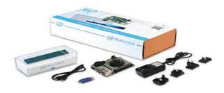
The development kit consists of a credit card-sized board and an Intel® RealSense™ camera (R200). Together, they help to bridge the gap between rapid prototyping and final product design.
