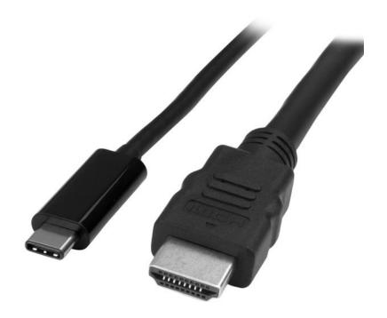
This USB- $C^{\text{TM}}$  to HDMI® adapter cable offers a convenient solution for directly connecting your DisplayPort over USB Type- $C^{\text{TM}}$  device to your HDMI monitor, television or projector. The adapter supports a connection distance of up to 1 m (3 ft.) and works with USB-C devices that support DP alt mode, such as the MacBook, ChromeBook Pixel<sup>TM</sup> and Dell<sup>TM</sup> XPS<sup>TM</sup> models 15 and 13. It's also compatible with Thunderbolt<sup>TM</sup> 3 ports.
