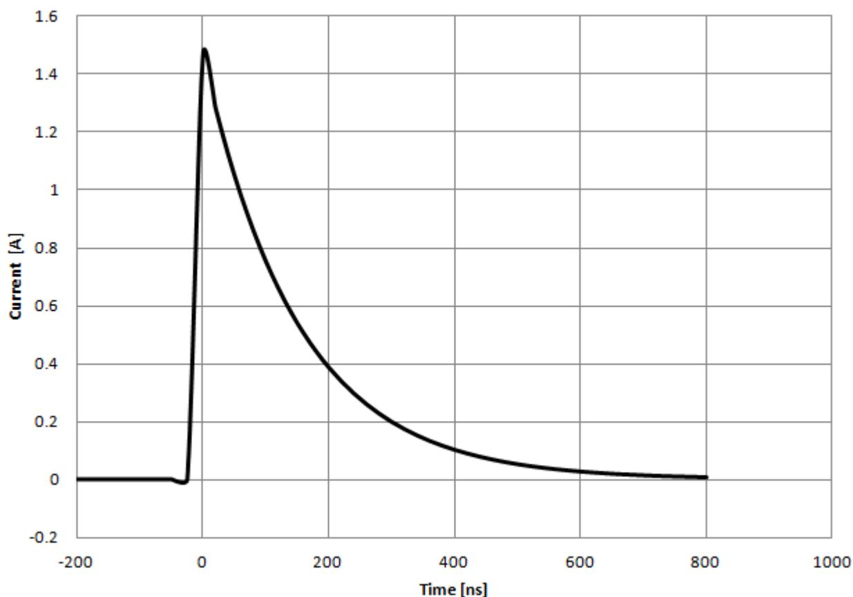
**Figure 2: A typical oscilloscope readout in a HBM test**
