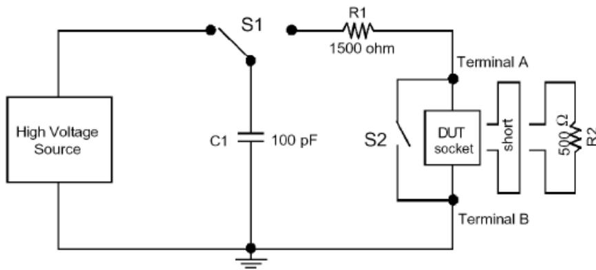
Figure 1: HBM test setup
