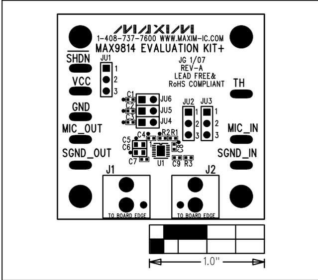
Figure 2. MAX9814 EV Kit Component Placement Guide—Component Side
