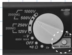
Protection against inadvertent setting of rotary switch to 1000 V rating
