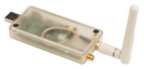
DC2274A-B SmartMesh IP USB Access Point Mote
