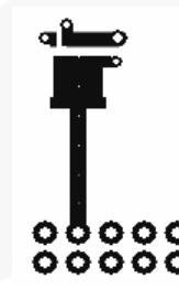
Figure 5. Minimum Pads of 2-ounce Copper
