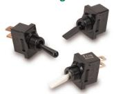
The D-Series single pole compact high current toggle switches are ideal for applications with back panel size constraints. These switches feature self-cleaning contacts and ratings up to 20A 125VAC, 10A 250VAC, 1 1/2 HP 125-250VAC. With an economical double insulated all-nylon construction, these switches figure prominently in the Environmental Controls, Marine, Food Service, Vacuum Cleaner and various other general purpose markets with stringent current carrying requirements.
