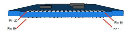
mangOH<sup>™</sup> PCB physical pinout
