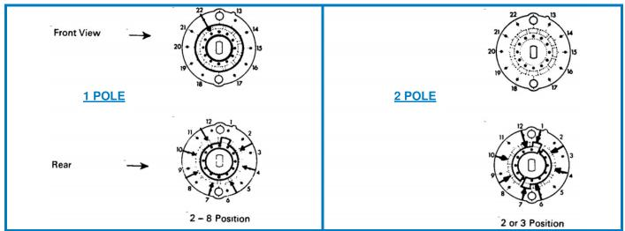
**Notes** Only available for 45° indexing with non-shorting rotor blades. Stops can only be fitted for 45° indexing at positions 3, 5 and 7.
