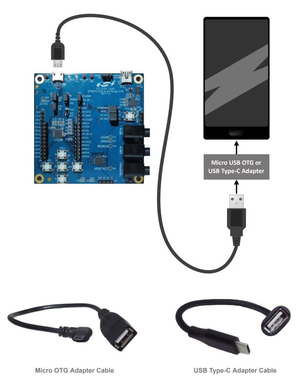
The Micro USB OTG adapter is for phones that use a micro connector. The USB Type-C adapter is for phones that use a USB Type-C connector.
