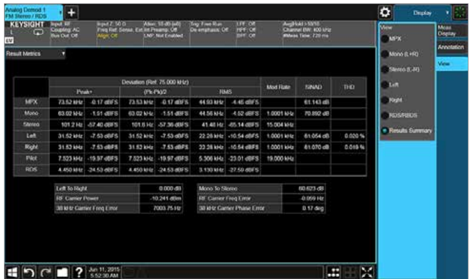
Figure 10. FM stereo numeric result metrics view/display with deviation, mod rate, SINAD, THD, left to right ratio, mono to stereo ratio and 38 kHz carrier frequency error, and phase error.
