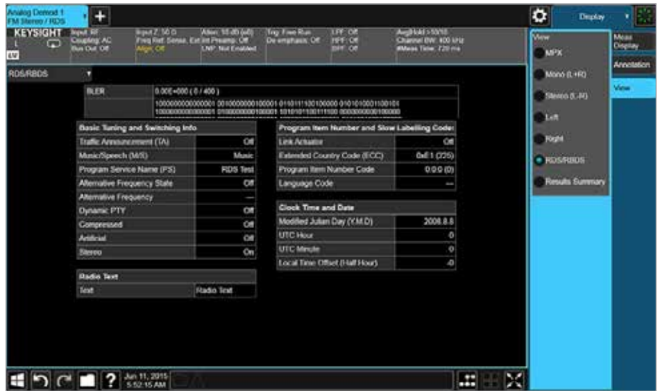
Figure 9. FM stereo RDS/RBDS decoding results view/display with BLER and decoded RDS information.
