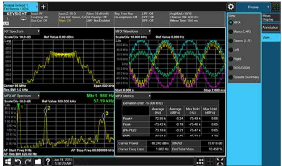
Figure 7. FM stereo MPX view/display with RF spectrum, AF spectrum, demod waveform and demodulation metrics results.
