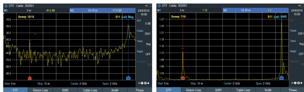
Figure 7-4: Distance to fault measurement
