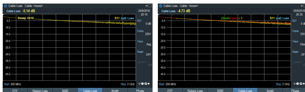
Figure 7-6: 1-port cable loss measurement
