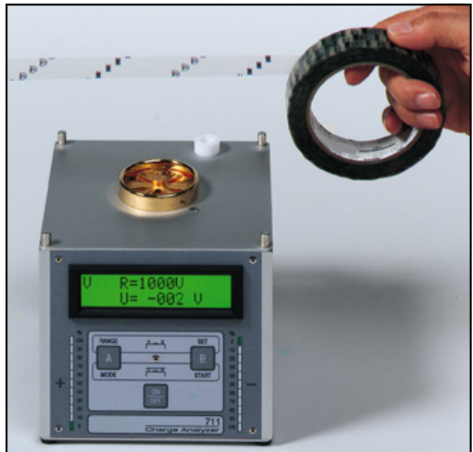
Figure 3. Testing Low Tribocharging Tapes.
