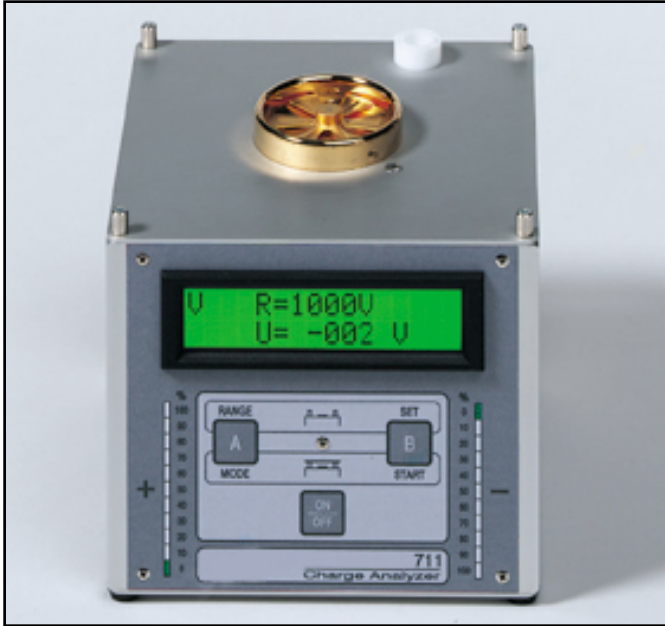
Figure 2. SCS 711 Charge Analyzer Field Meter Operation.
